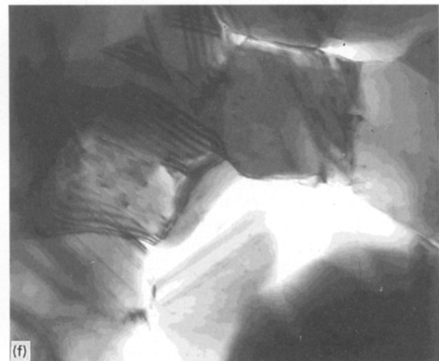
Figure 6 TEM images for the microstructure of the copper films. Deposition temperature; (a, b) 145 °C, (c, d) 231 °C, (e, f) 317 °C.
